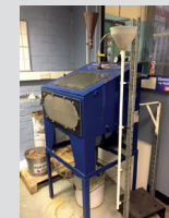
◀ Sand Erosion Cabinet for testing to MSRR9910 Test 22 with separate ASTM D968 Sand Abrasion tester.
