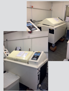
Salt Spray Cabinets for testing to ASTM G85 and Annex 1,2,3 and 5. ▶
