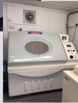
◀ Salt Spray Cabinets for testing to ASTM B117.
