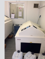
▶ 100% Humidity Cabinet for testing to ASTM D2247 or BS3900 F9.
